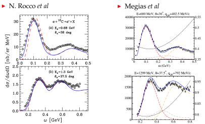
★ Mechanisms other than single nucleon knock-out and leading to the appearance of 2p2h final states (ground state correlations, final state interactions and coupling to MEC) play a significant role
