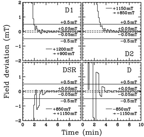
Figure 2: Typical magnetic field responses of the dipole magnets D1, D2, and DSR of Grand Raiden, and the magnet D1 of Large Acceptance Spectrometer.
