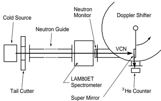
Figure 1. Experimental setup for UCN measurement.
