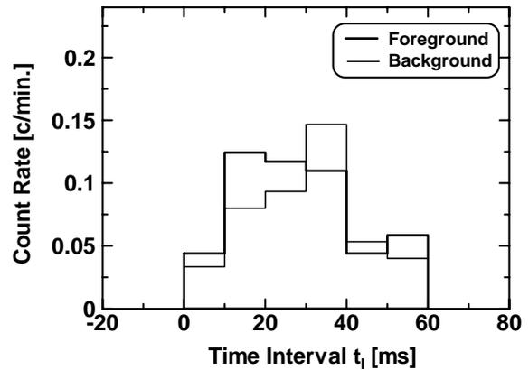
Figure 2. Distributions of  $t_i$  obtained for the foreground (thick histogram) and background (thin histogram) measurements.
