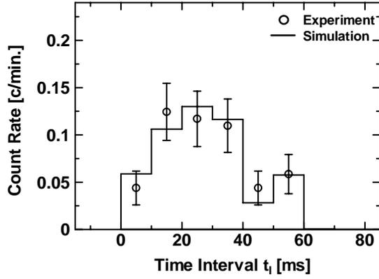
Figure 3. Comparison between the measured (circle) and calculated (histogram) distributions of  $t_l$  for the foreground.
