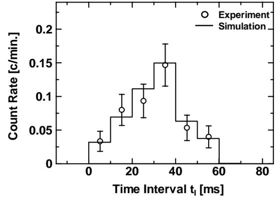
Figure 4. Comparison between the measured (circle) and calculated (histogram) distributions of  $t_l$  for the background.
