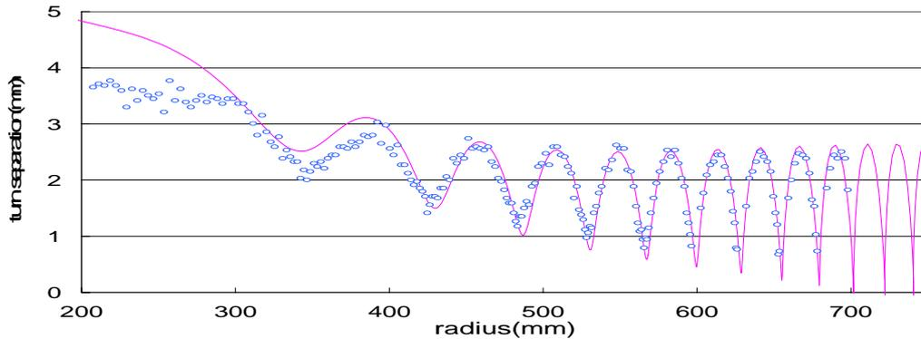
Figure 2: Observed (circle) and calculated (line) turn separations as a function of a radius.
