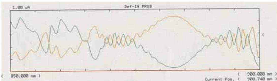
Figure 1 65MeV Proton beam currents as a function of a position of the beam probes
