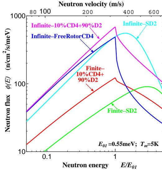
Figure 2: Calculated results of VCN spectra for typical cases of CD<sub>4</sub> and ortho-D<sub>2</sub> moderators. (Neutron flux is normalized to the source intensity corresponding to the specific loss rate of 1 n/cm<sup>3</sup>/s.)
