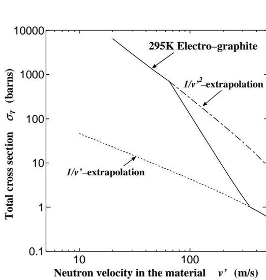
Figure 1: Measured total cross section  $\sigma_T$  in VCN region for electro-graphite [3] (solid line) versus neutron velocity  $v'$  within the material.
