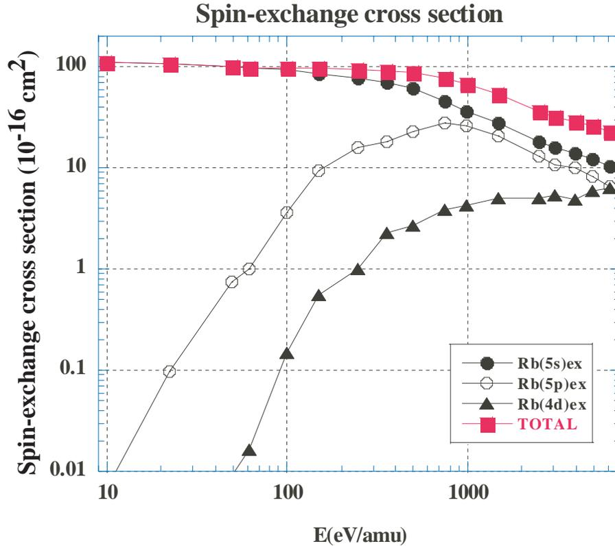
Fig. 2. Calculated energy dependence of the spin-exchange cross sections for  $\text{Li}^{2+} + \text{Rb}$  system.
