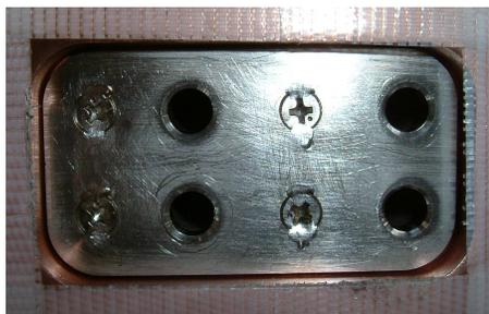
Figure 1: Stainless steel plate covering welds.
