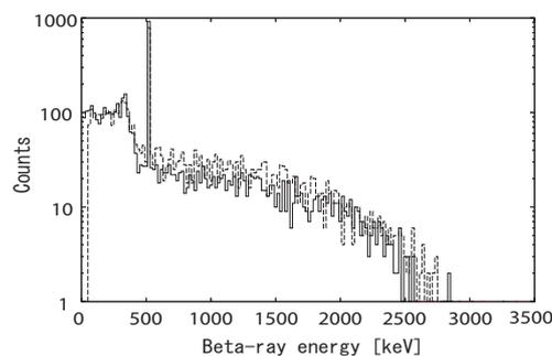
Figure 1: Beta-ray spectra of  $^{98}\text{Rh}$   $\beta$  decay feeding the  $2^+$  state at 652 keV in  $^{98}\text{Ru}$  obtained in this experiment (dashed line) and by the GEANT4 simulation (solid line).
