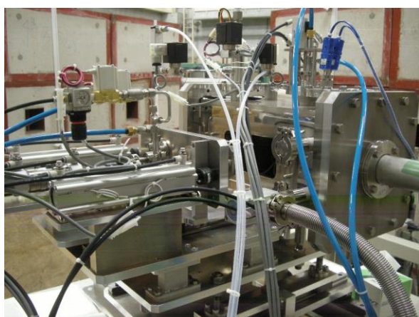
Figure 2: Irradiation chamber for RI production placed at the end of F-course in M-exp. room.
