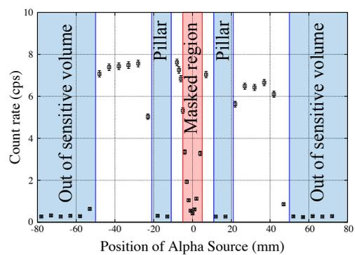
Figure 4: Counting rate of the  $\alpha$  particles emitted from the  $\alpha$  source as a function of the position of the source.
