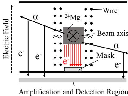
Figure 1: Schematic view of the insensitive volume introduced by the mask.
