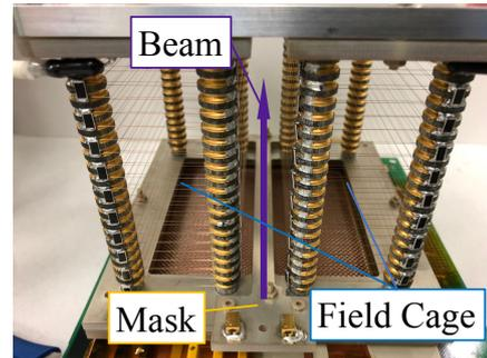
Figure 2: Picture of the TPC with the mask. A beam passes through the center of the TPC along the solid arrow. The mask is installed along the beam trajectories.
