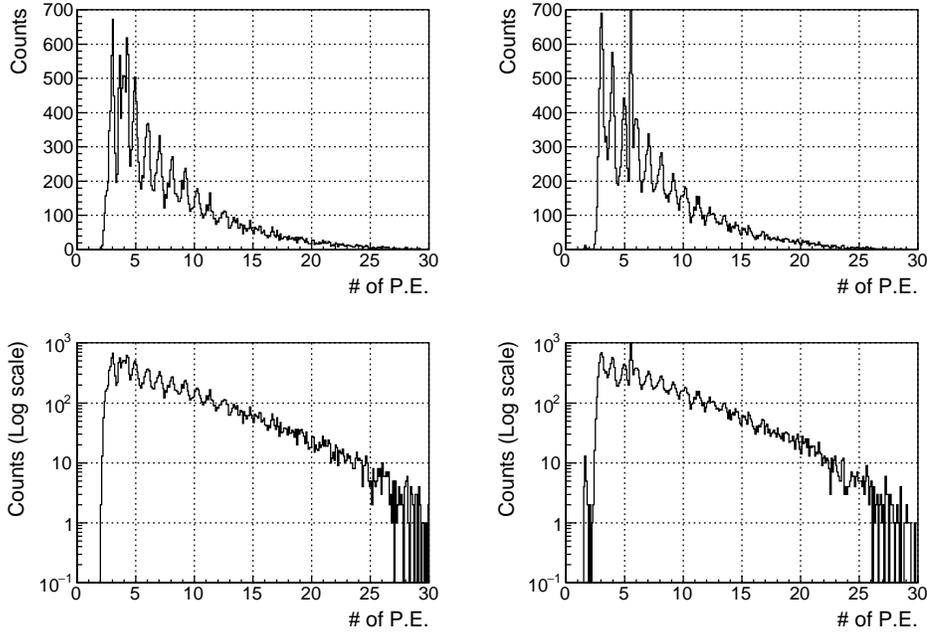
Figure 3: Distributions of number of p.e. of both top (left) and bottom (right) edge of the test Cherenkov timing detector with SBD. Top and bottom figure show normal and logarithmic scale of the vertical axis, respectively. Spike noises on the DRS4 waveform data are shown as a peak structure around number of p.e. of 5.
