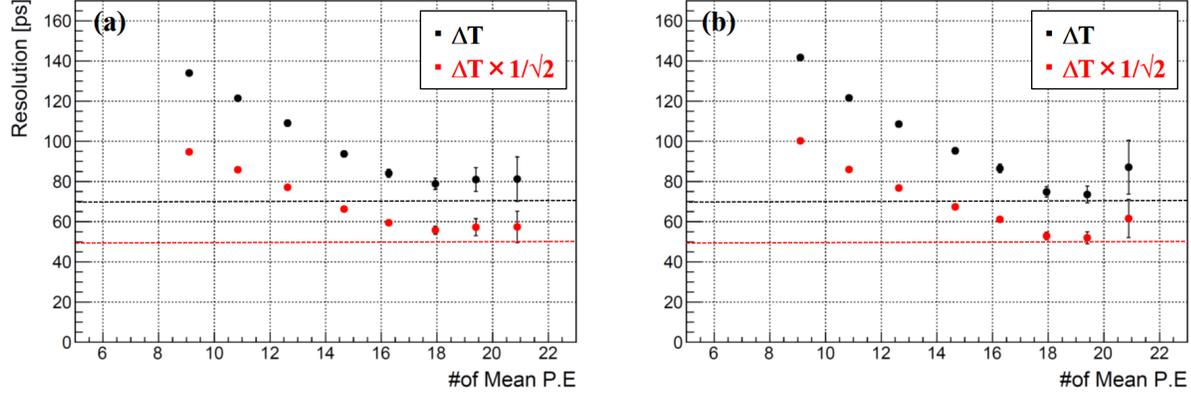
Figure 5: Time resolutions by selecting number of p.e.. (a) and (b) show the resolutions by correcting the time-walk by information of the pulse height with filtering by SBD and the signal width with both filtering by SBD and the integration, respectively. Black and red points show the measured and estimated (divided by  $\sqrt{2}$  of measured values) time resolutions, respectively. Time resolution of 70 ps and 50 ps are indicated by black and red dashed lines, respectively.
