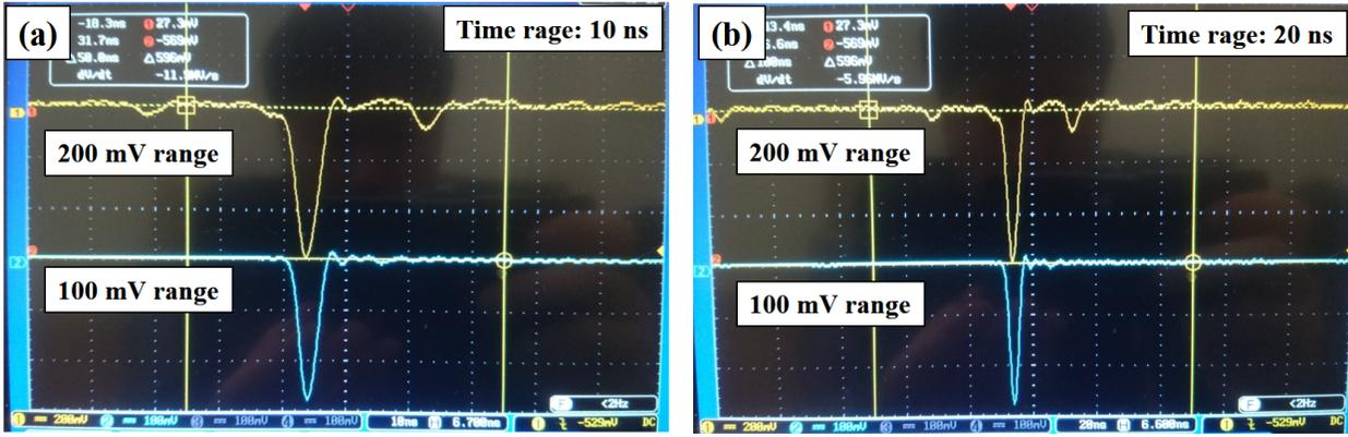
Figure 1: Oscilloscope snapshots of output signals before and after filtered by SBD. Channel 1 (yellow line) and channel 2 (blue line) show output signals before and after processed by SBD, respectively. (a) and (b) show different time ranges of 10 ns and 20 ns, respectively.
