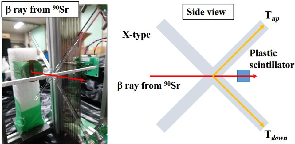
Figure 2: Photograph of the test Cherenkov timing detector (left). Time resolution of the detector was evaluated by using a  $\beta$  ray from a  $^{90}\text{Sr}$  source. The time difference between both edge ( $T_{up}$  and  $T_{down}$ ) of the detector was measured.
