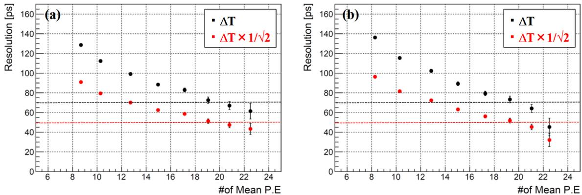
Figure 4: Time resolutions by selecting number of p.e.. (a) and (b) show the resolutions without and with SBD, respectively. Black and red points show the measured and estimated (divided by  $\sqrt{2}$  of measured values) time resolutions, respectively. Time resolution of 70 ps and 50 ps are indicated by black and red dashed lines, respectively.
