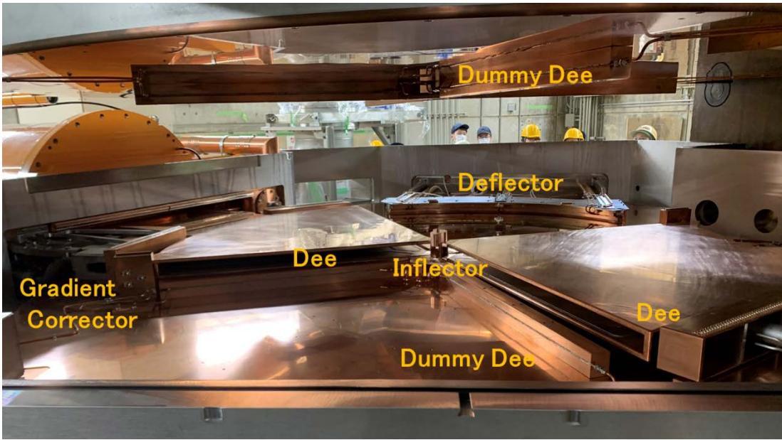
Figure 1. Photograph of the inside of the vacuum chamber of the AVF cyclotron with the upper yoke lifted by the renewed yoke lifter.
