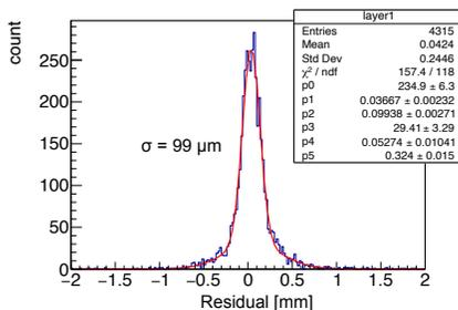
Figure 2: Spatial resolution of the drift chamber measured with the proton beam in the performance test.
