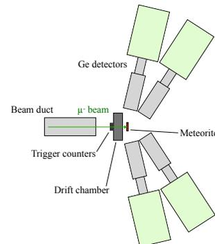
Figure 3: Schematic view of the proposed 2d imaging system for muonic X-ray analysis.
