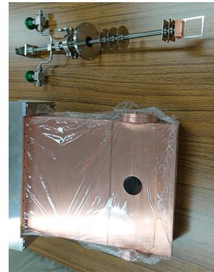
Figure 4: Photograph of a newly designed sample chamber and sample holder.
