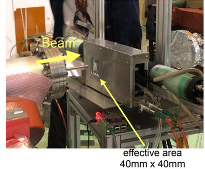
Figure 1: Photograph of newly developed tracking drift chamber taken in the test experiment with the proton beam.
