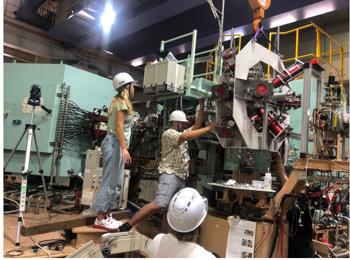
Figure 3: Left panel: a gamma-ray detector array SC \gamma LLA [10] using eight large-volume LaBr 3 (Ce) detectors [12, 13] was modified to accommodate the PANDORA scattering chamber at the center. Right panel: a picture during the placement of SC \gamma LLA at the target position.
