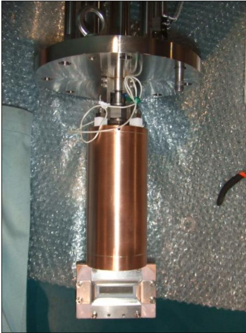
The gas cell for inelastic measurement
