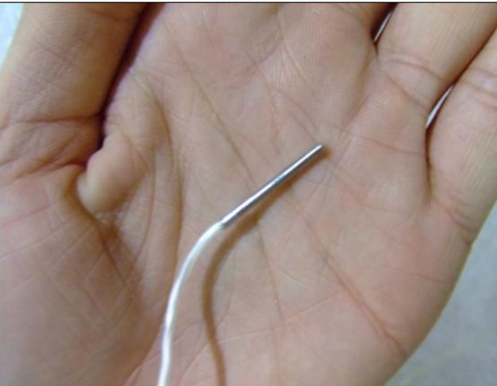
A pt-100 temperature sensor made by CHINO (model no. R610-3)
