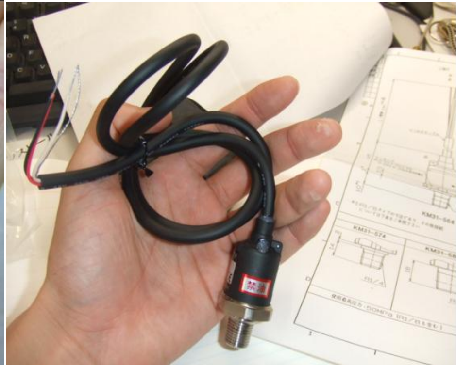
A pressure transmitter made by NAGANO-KEIKI (model no. KM31)
