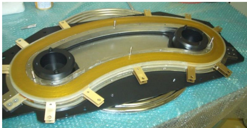
Three double-pancakes and cooling plates are stacked and fixed with epoxy resin in vacuum.
