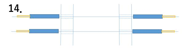
New feed-throughs are set to the through holes with glues.
