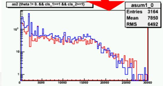
Fig.4: ADC spectrum with  $V_{gem}=410$ (blue),  $417$ (red)V
