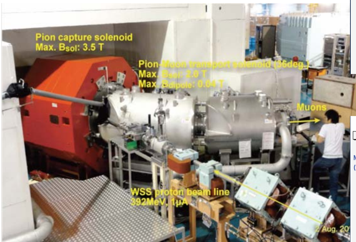
Figure 2: Solenoid and muon transport system
