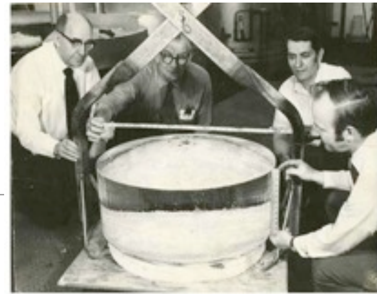
The first 32 inch diameter NaI(Tl) crystal. Pictured from left to right are Dr. Swinehart, Ed Jablon, Joe Knaus and Marko Stigoi.
