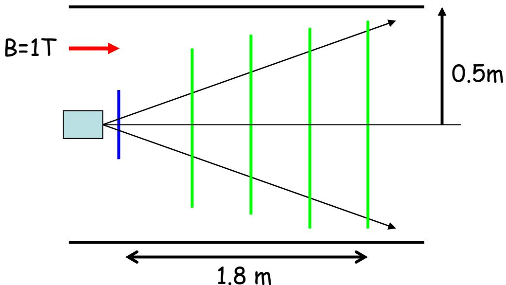
$\sigma_{xy} = 150\text{um}$ ,  $N=13$ ,  $P=1\text{ GeV}/c$
