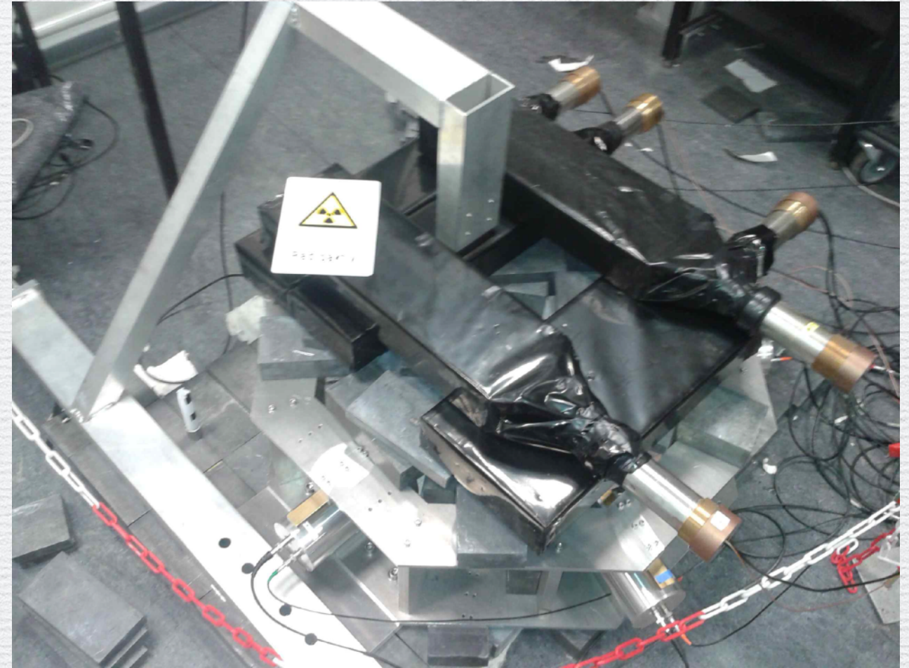
Figure 3.4: The setup shown in Fig. 3.3 was covered with a 5-10 cm thick layer of lead (left-hand side). Five plastic scintillators were positioned on top of it to veto background events (right-hand side).
