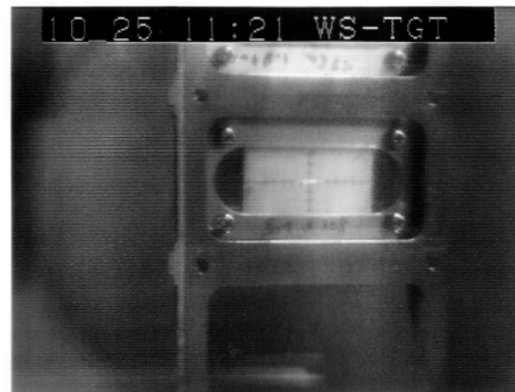
Beam spot in the dispersive mode
