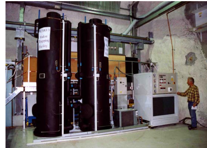
Free-Radon Air Factory (15Bq/m 3 → <15mBq/m 3 )
