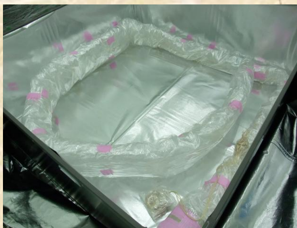
Air-tight bag filled with N 2 gas
