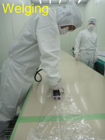
Balloon made by welding
