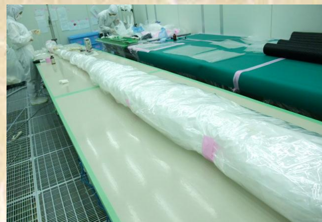
Balloon is covered by protection film
