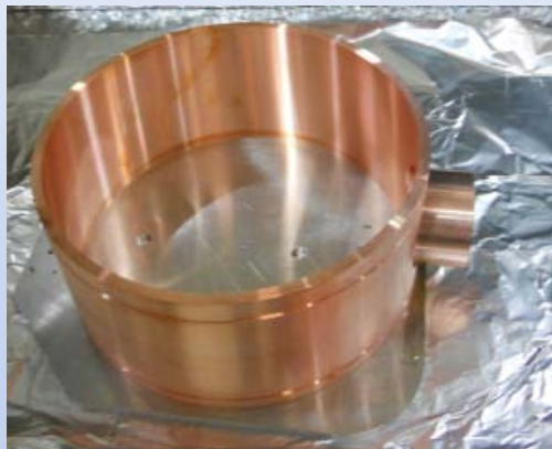
Demonstrated e-beam weld for cryostat hoop
