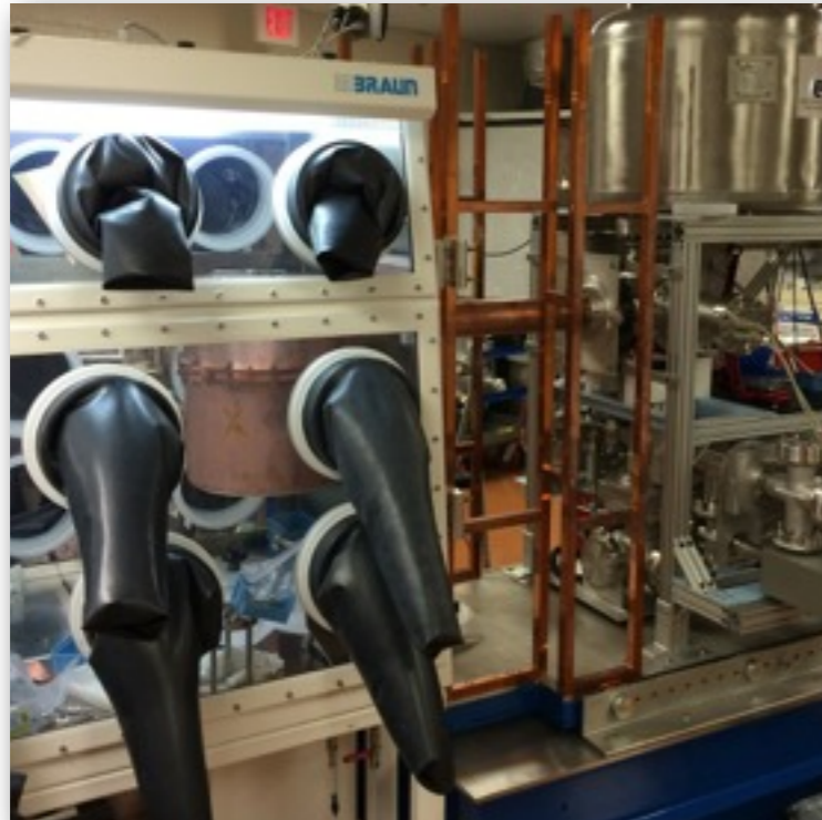
Cryostat mated to the glovebox for string installation
