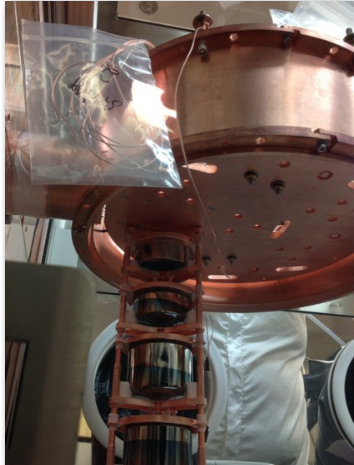
First string of ^{enr}\text{Ge} in Cryostat 1
