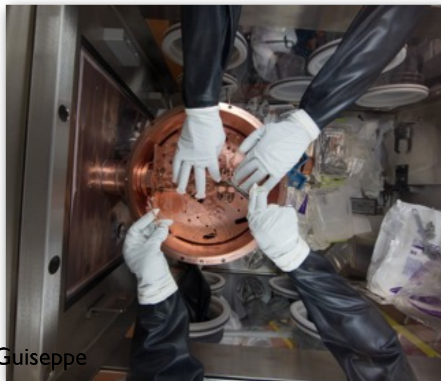
Cryostat mated to the glovebox for string installation
