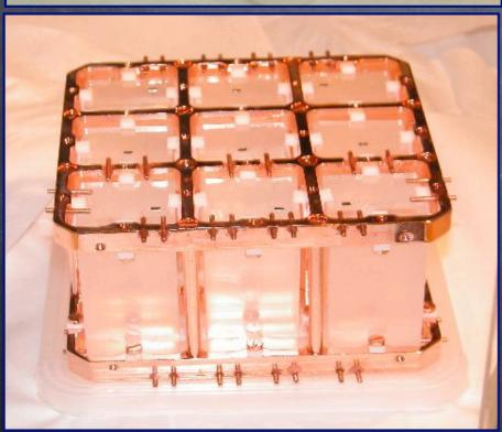
The bulk of Cuoricino calorimeter is made by 44 TeO<sub>2</sub> crystals of 5x5x5 cm<sup>3</sup> (790 gr of weight).
