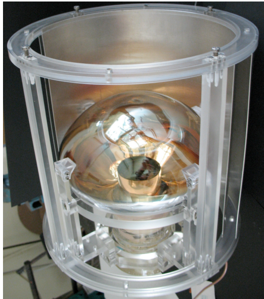
Magnetic Shield Support Structure Spain
