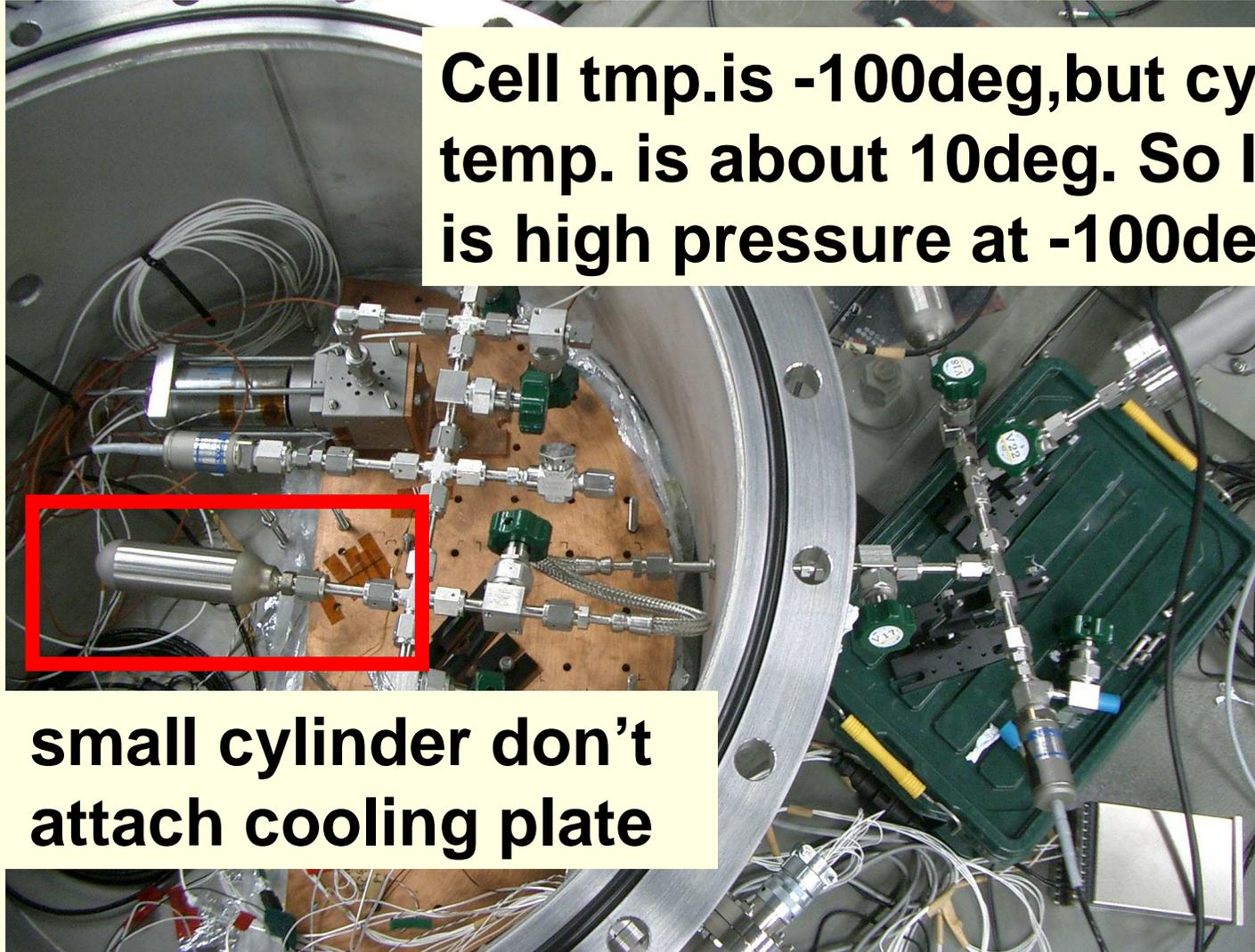
**small cylinder don't attach cooling plate**
