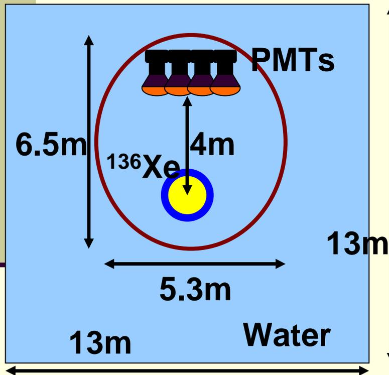
Water shield and ELT reduce gamma rays from rocks and PMTs.
