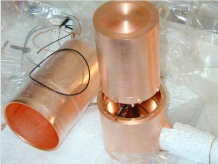
Low-background detector and electroformed cryostat during assembly
