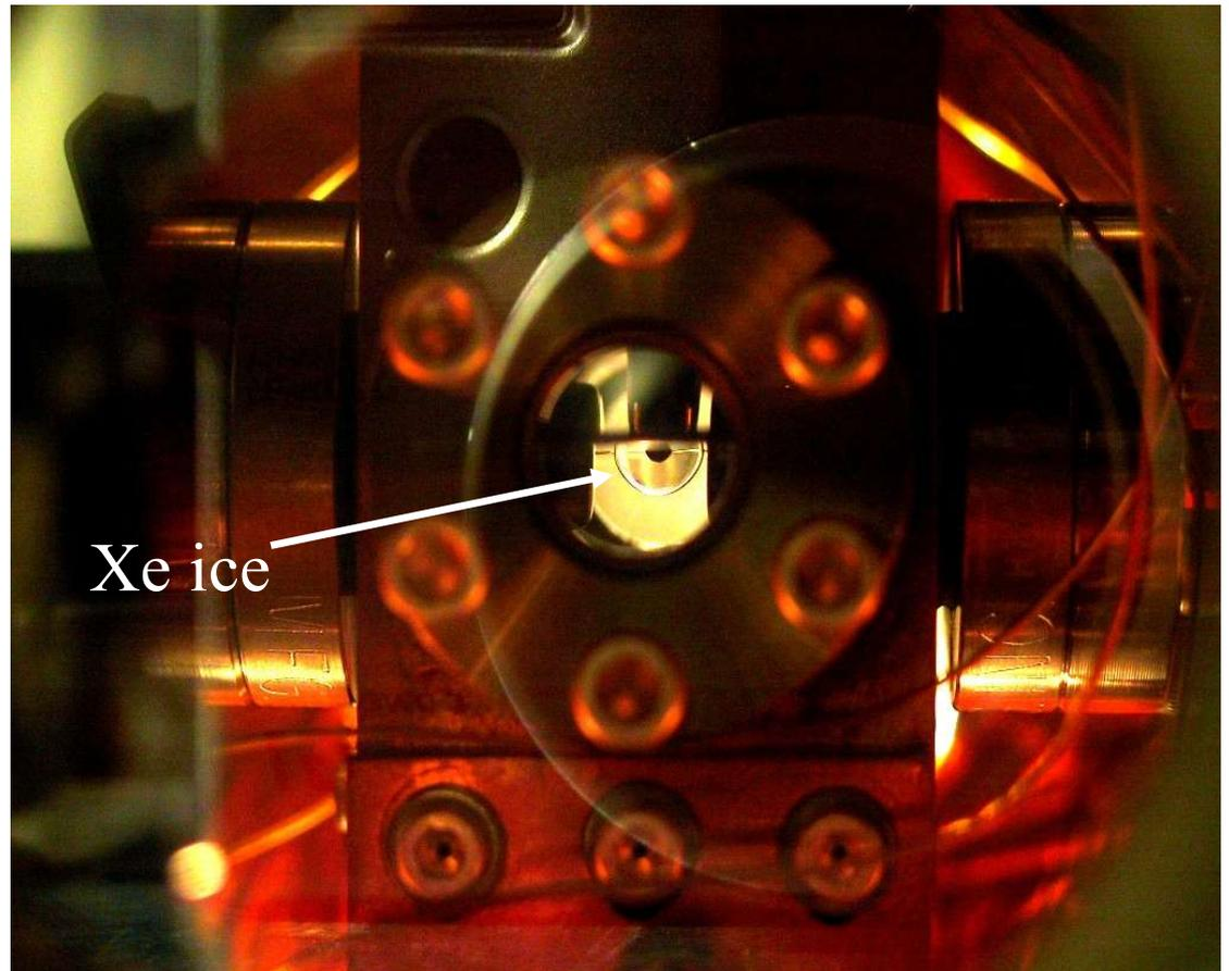
**Cold probe has demonstrated ion capture in ice and release through melting.**
