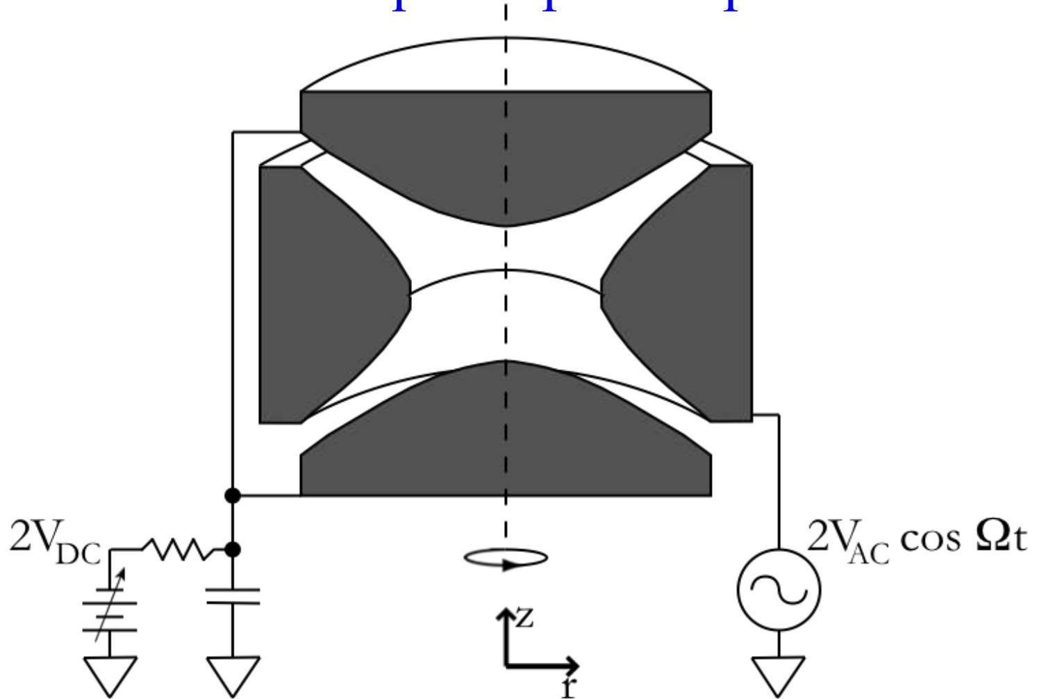
RF voltage confines ions to the center of the electric pseudo potential given by  $\psi \sim |E|^2$ .
