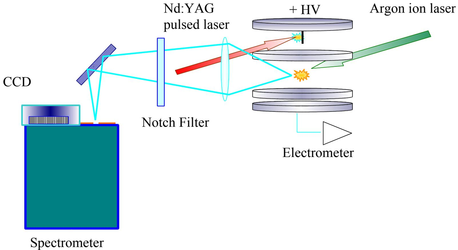
Whole fluorescence spectrum can be measured in one laser shot
