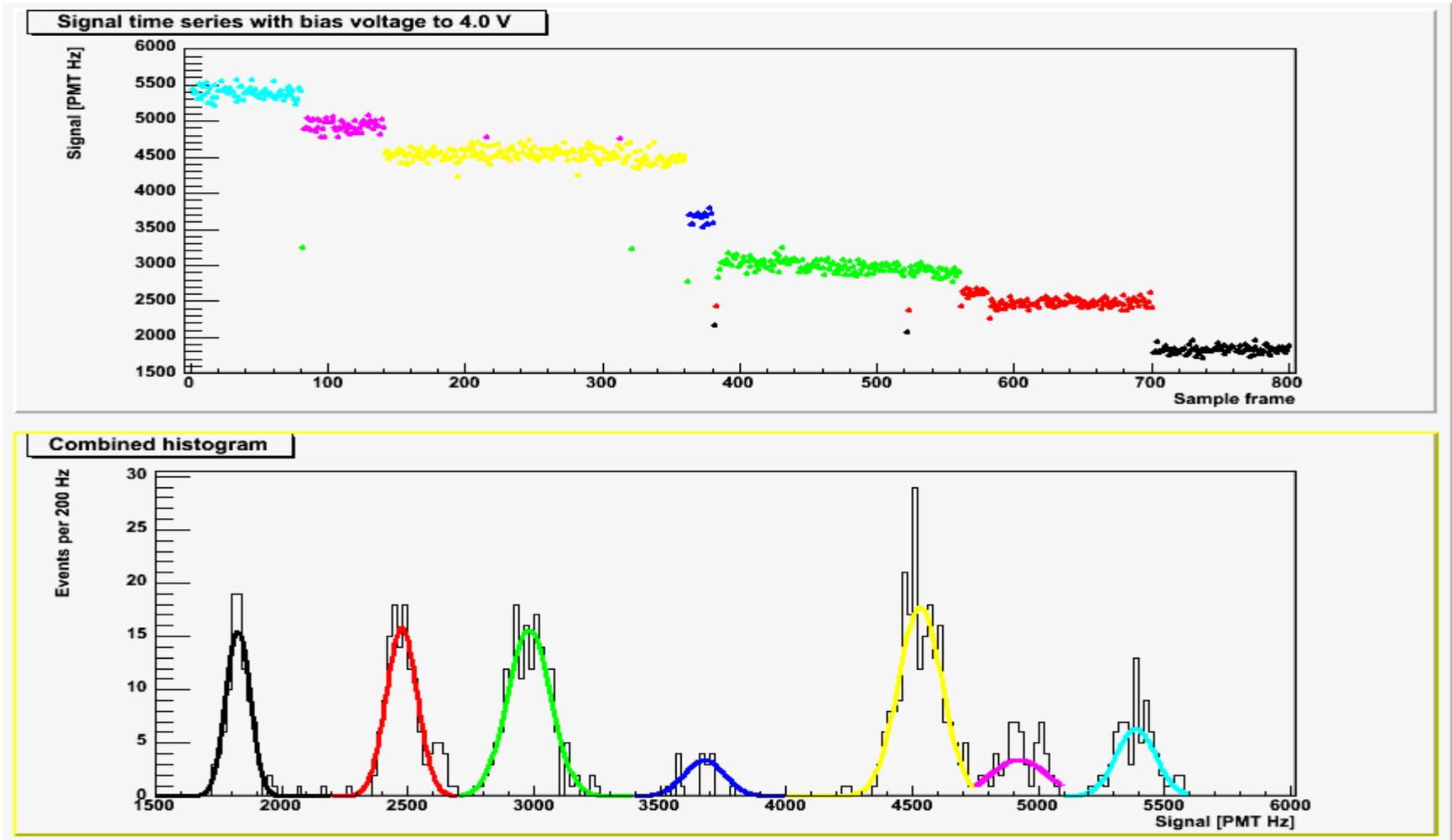
Quantization of PMT signal demonstrates single ion sensitivity
